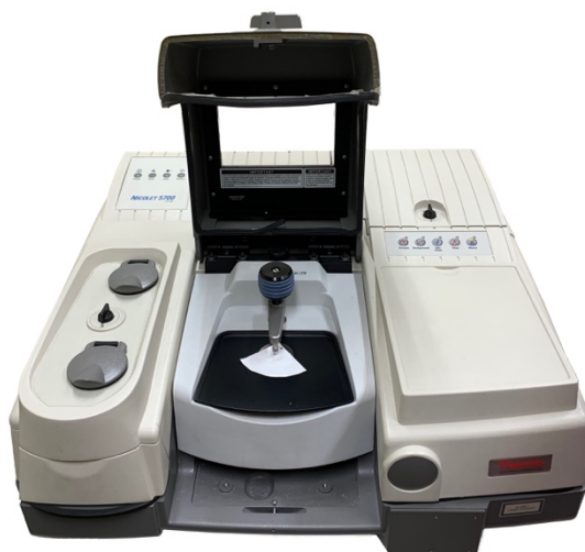
Figure 11. Photograph of the Nicolet 5700 FT-IR spectrometer with Golden Gate MKII ATR accessory.
